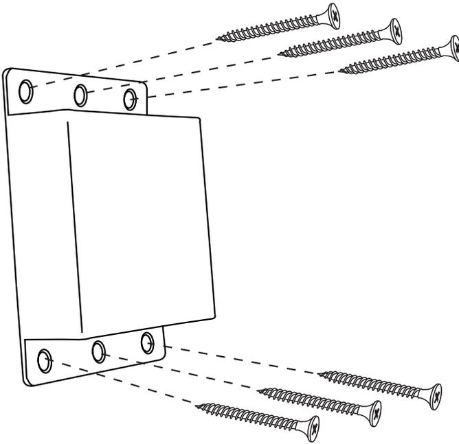
The Gefen *DisplayPort Extender over CAT-7* can be mounted on any horizontal or vertical flat surface (e.g. wall or inside / outside a cabinet with wood / drywall screws) as shown in the diagram above. There should be an inch or two of clearance between the edges of the unit and any walls or vertical surfaces to allow for enough clearance for connection and disconnection of the DisplayPort cable.
