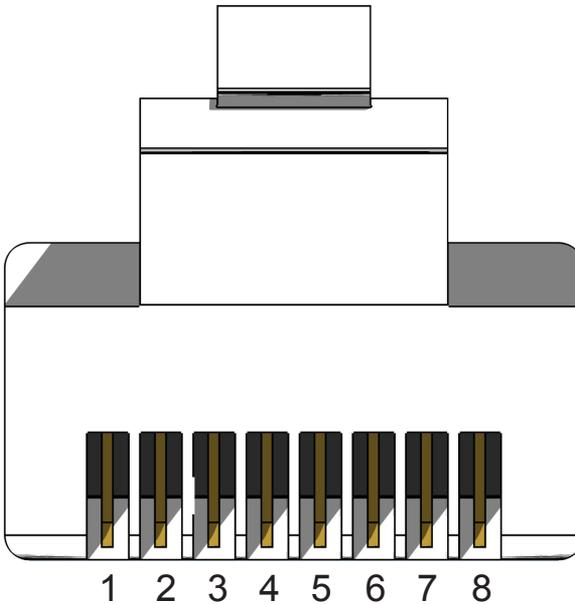
Gefen recommends the TIA/EIA-568-B wiring option. Use the table below when field-terminating cable for use with Gefen products.
