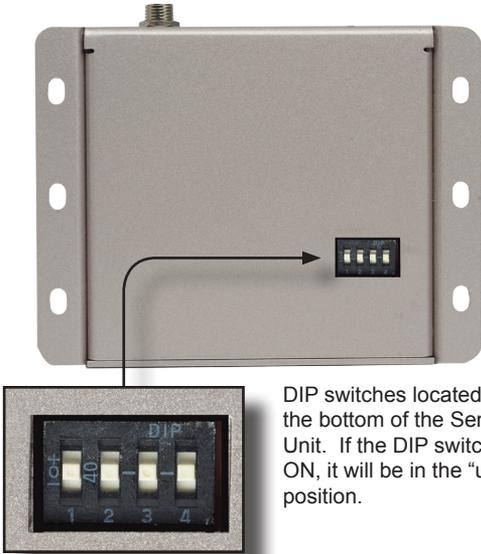
DIP switches located on the bottom of the Sender Unit. If the DIP switch is ON, it will be in the “up” position.
